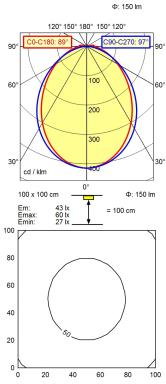
light sourceLEDwork equipmentwithoutconnected load22-26 V, DCpower consumptionenv. 3,0 Wluminous fluxapprox. 150 lmluminous efficiencyapprox. 50 lm/W
